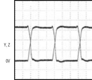
UNLOADED DRIVER OUTPUT WAVEFORM (f IN = 16Mbps)
